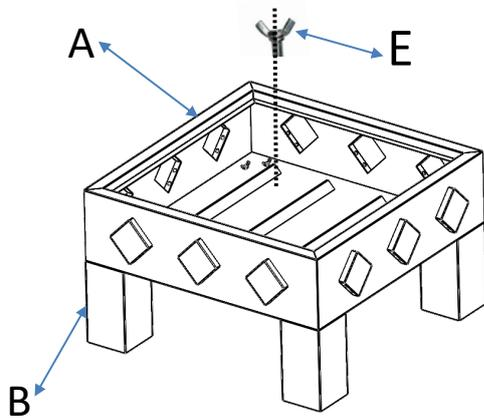
Connect the fire bowl (A) and four legs (B) with screws (E)
