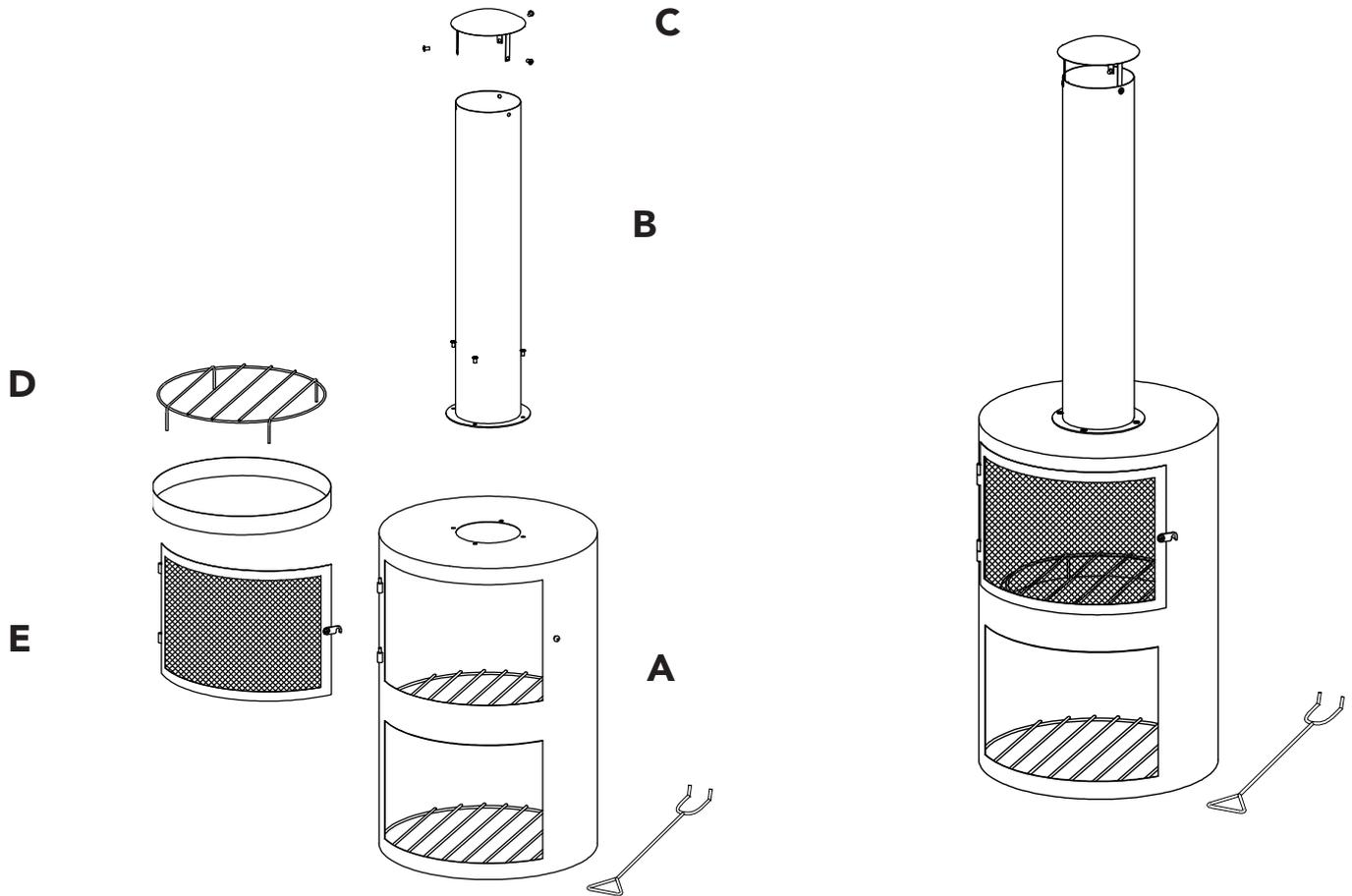
**Step 1:** Connect the Base (A), the chimenea (B) and the raincap with the bolts and nuts.
